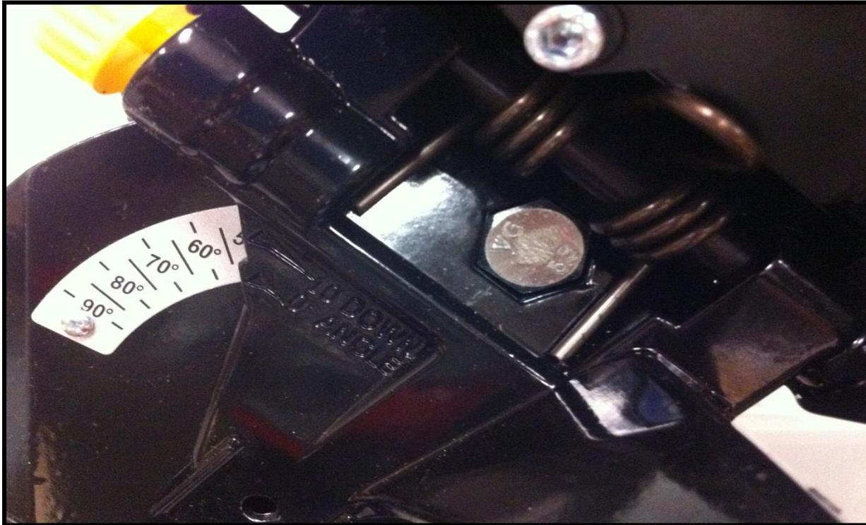
***Set the grinder head angle to the manufacturers recommended Top Plate Sharpening Angle. Position the “0” reference mark on the angle desired when sharpening chains without “down Angle”. Position the “10 down” reference mark when sharpening chains with “down angle”.***
