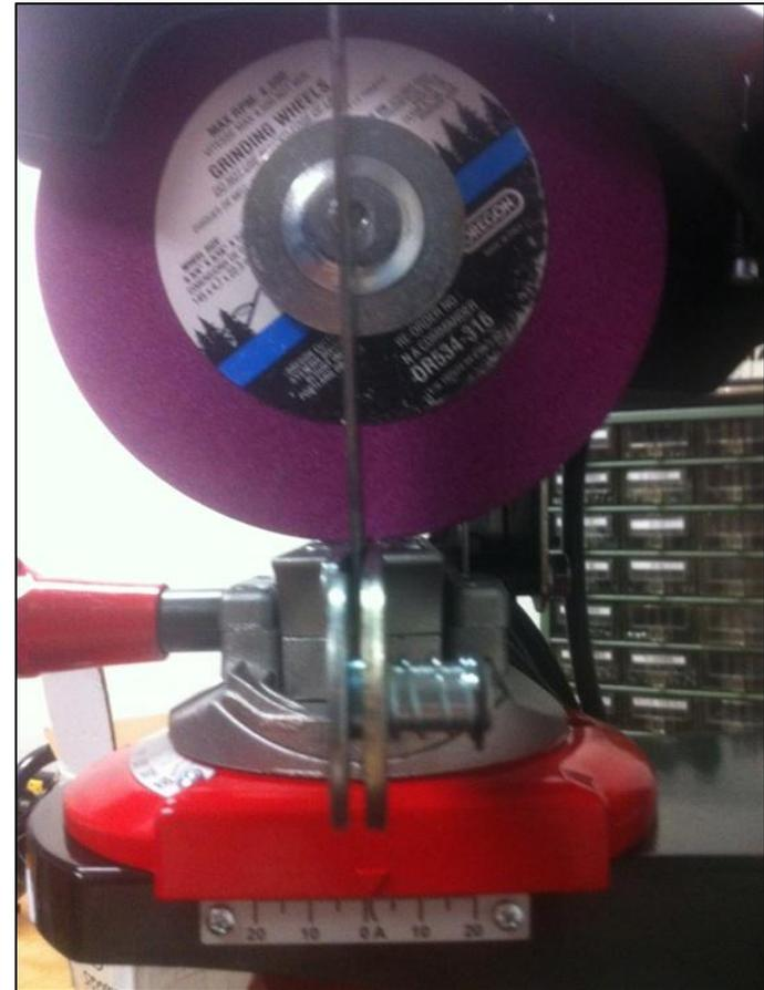
Pull the grinder head down until the grinding wheel touches the chain vice. Check the alignment between chain vice and center bolt attaching the grinding wheel.
