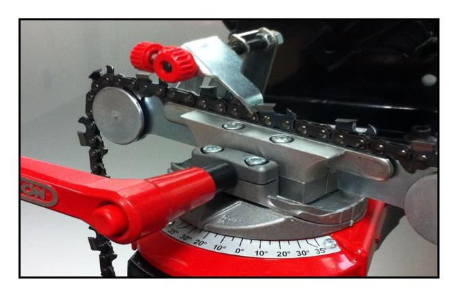
Set the vise assembly to the manufacturers recommended top plate sharpening angle for your chain by loosening the knob and turning the vise clockwise for RH cutters counter clockwise for LH cutters.
