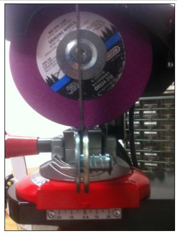
Pull the grinder head down until the grinding wheel touches the chain vice. Check the alignment between chain vice and center bolt attaching the grinding wheel.
