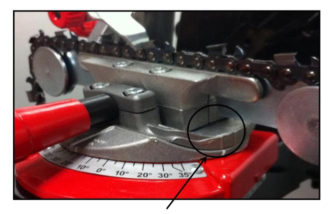
Tip: Push the knob away "right away" from the operator for RH cutters until the raised line closest to the operator lines up with the triangular indicator on the vise base. Pull the knob towards operator for LH cutters, until the line furthest from the operator lines up with the triangular indicator on the vise base
