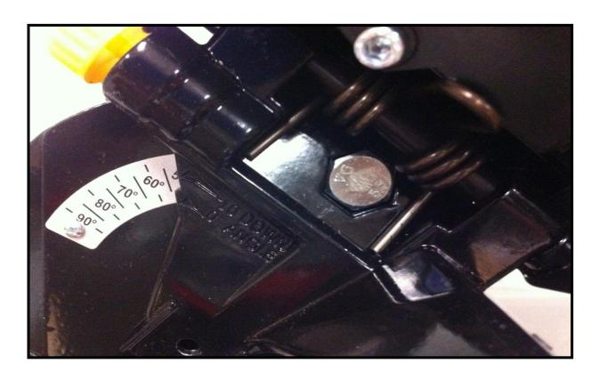
Set the grinder head angle to the manufacturers recommended Top Plate Sharpening Angle. Position the "0" reference mark on the angle desired when sharpening chains without "down Angle". Position the "10 down" reference mark when sharpening chains with "down angle".
