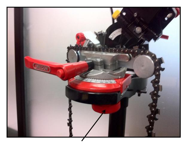
Loosen the knob and tilt the vice away from the operator for RH cutters. Tilt the vice towards the operator LH cutters.
