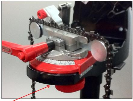
To move the chain vice assembly loosen the two 4mm Allan head bolts located under the chain vice. These bolts are located on each side of the "Red" adjustment knob.
